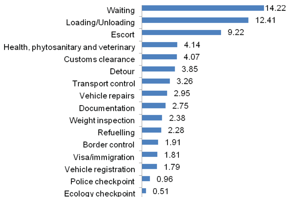
Figure 5: Average duration of road activities (hours) per 500 kilometers
